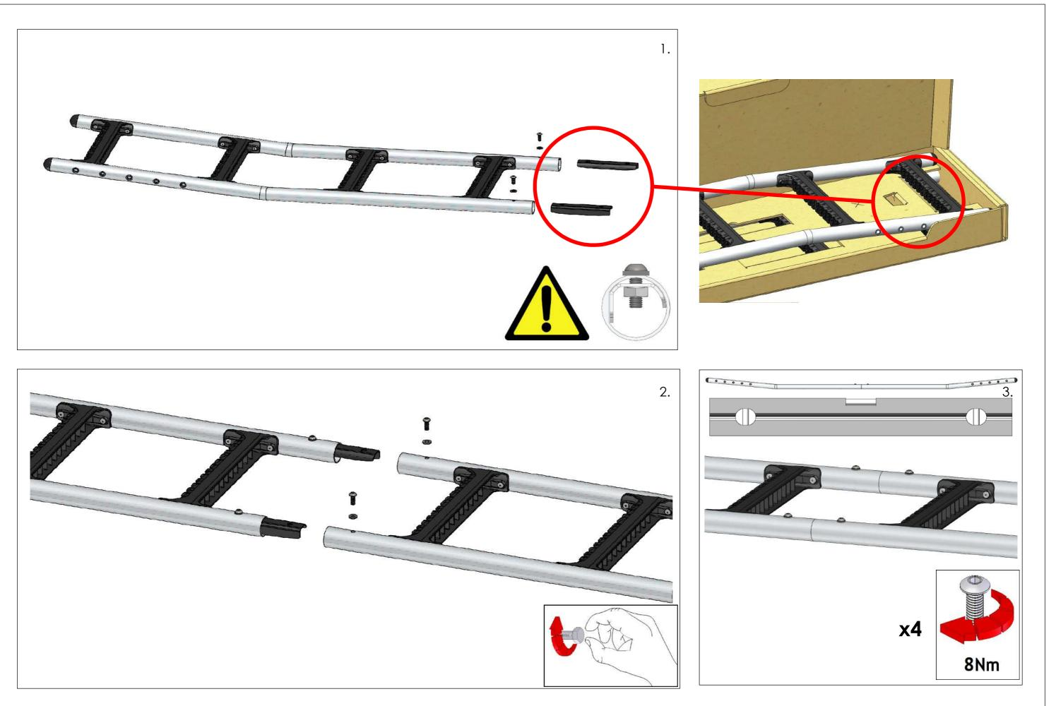
LK42\_a Aluminium Ladder Fitting Kit, Deliver 9 - H2/H3
